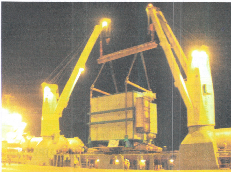
Boiler being loaded on mv Annette
